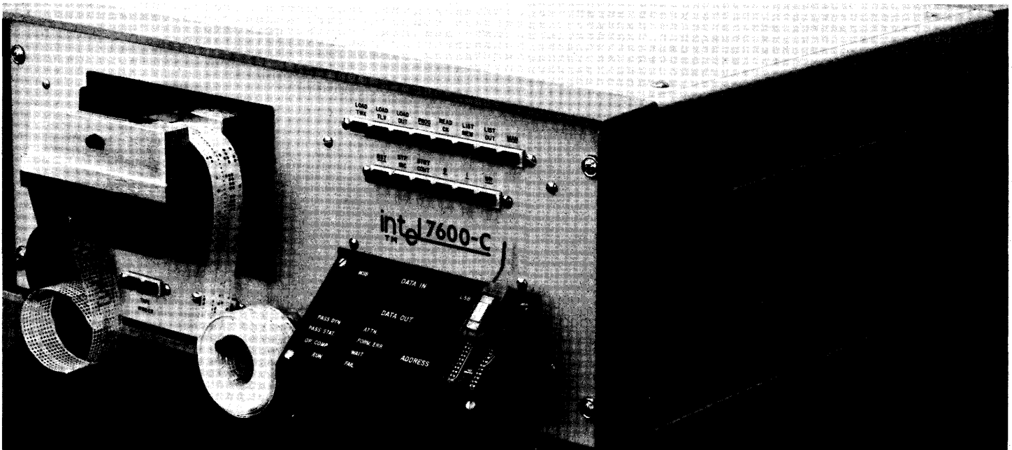
Fig. 1. Photograph of ROM Programmer Using MCS-4
